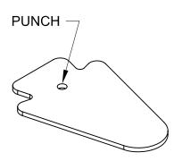
STEP 5: USING THE ARROW HEAD AS A GUIDE, PUNCH A HOLE IN THE STRAP AND SECURE WITH LONG RIVET.
