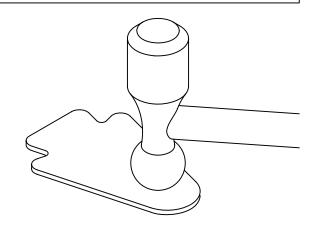
STEP 3: USING THE SHORT RIVET, INSERT INTO THE STRAP AND PEEN FLAT. (RIVET FROM THE BACKSIDE)
